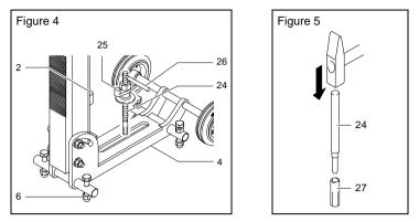
Align the drill stand plate (4) on the drillhole to be drilled of the wet diamond drill bit:
